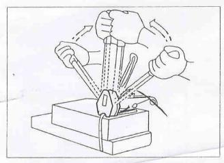
5. Open the sealer fully open position, place the sealer on the top of the seal, press the handle together to fully crimp the seal, remove the sealer.
