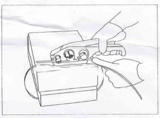
1.Place the strap around container as shown, take the tensioner in your right hand and depress the tension lever, place the strap under the gripper and the bottom section of cutter housing, the end of strap should protrude 2" beyond the tool, release the tension lever.
