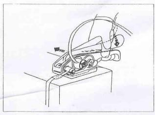
Depress the tension lever to cut the strap, with the tension lever depress pivot the tool to the right, and remove from the completed strap.
