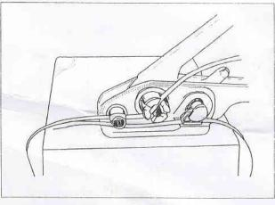
2. Slide the top strap into the cutter slot and the windlass slot.
