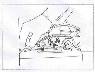
4. When proper tension is reached, place the seal open side down over both straps in front of the tool.
