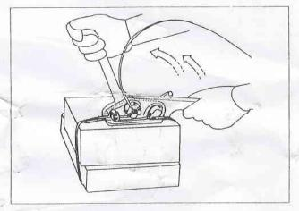
3. Hold the tool with your left hand and move the handle hack and forth with your right hand,until the strap is tensioned.
